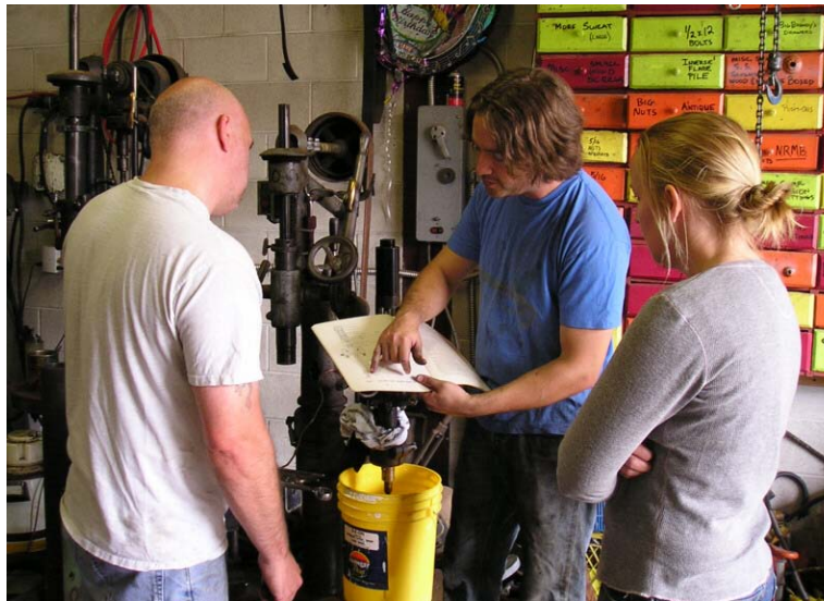
The Diesel Engine Theory Workshop uses an original Washington Iron Works engine manual to set the injector spring tension
