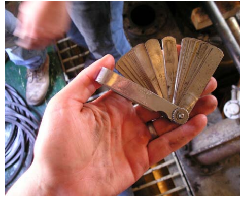
Feeler gauges, used to take precise measurements
