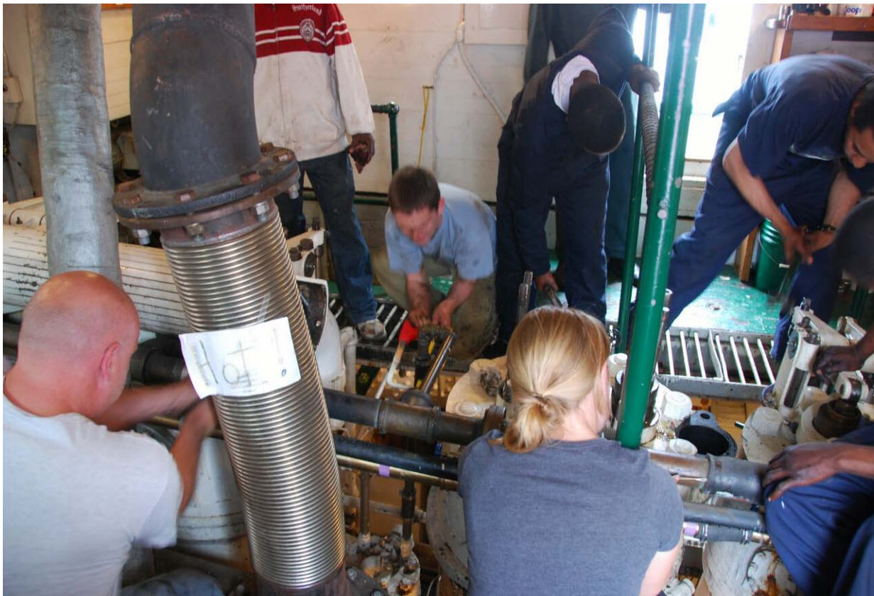
Participants in the 2009 Diesel Engine Theory Workshop disassemble components of the cylinder head and air manifolds, using wrenches, sockets, vice grips, and other standard tools
